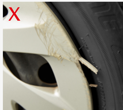
Cracked wheel trim
