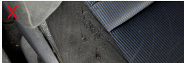
Excessive wear or rips in upholstery
