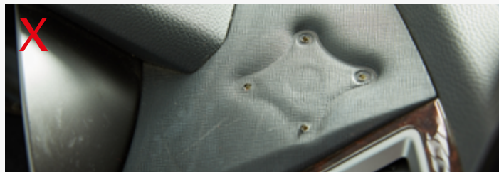
Holes in trim
