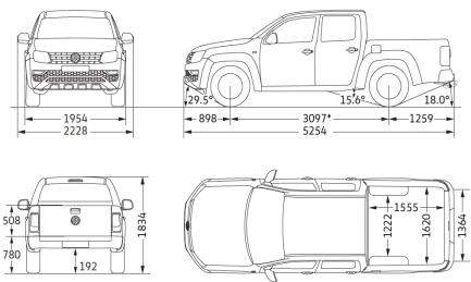
\*This value applies for unladen weight. When loaded, the wheelbase is 3,090 mm.
