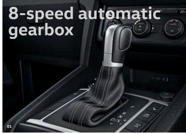
01 Optional 8-speed automatic gearbox and permanent 4MOTION all-wheel drive. The new Amarok is the only vehicle to offer the unique combination of comfortable 8-speed automatic gearbox with the iconic torsen differential and permanent 4MOTION all-wheel drive. The first gear is designed for off-road driving, whereas the eighth gear is optimised for economical driving at low engine speeds.
