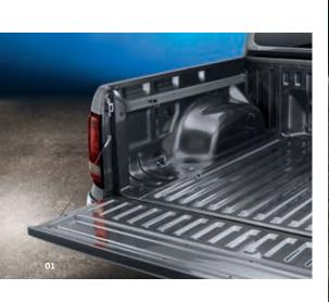
The smoothest moving tailgate. It can be loaded with up to 200 kg and can serve as a load platform extension.
