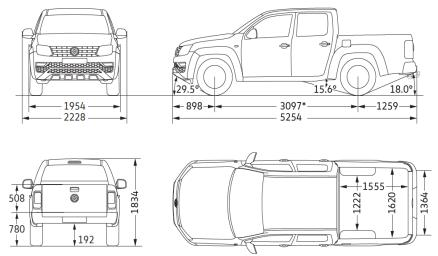
\*This value applies for unladen weight. When loaded, the wheelbase is 3,090 mm.
